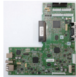
A printed circuit board for a printer
